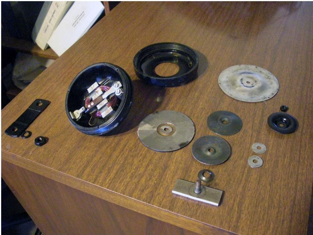
Mounting strap with nut and washer, bakelite housing with coils and breaker, bakelite closing ring, tympani, contact bar, conical washer, compression discs, two spacer washers, tympani cover plate, front disc, and nut.
