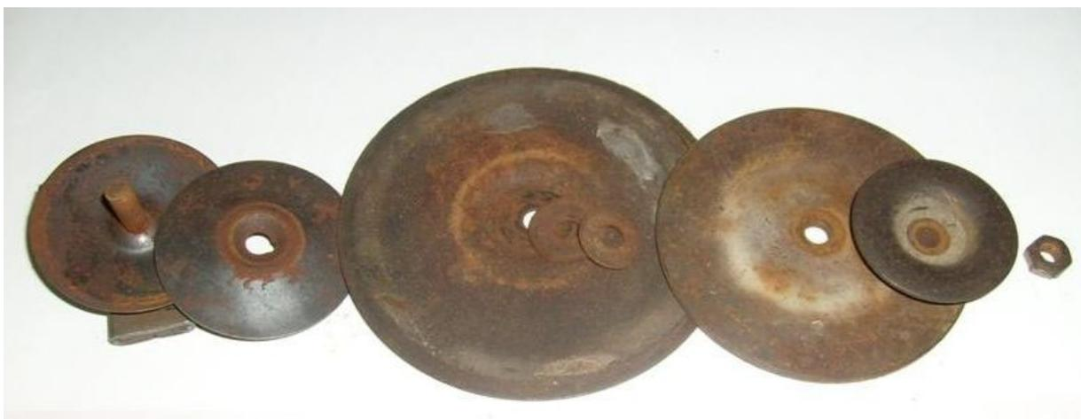
Contact bar with conical washer and first compression disc (shown assembled), second compression disc, tympani, two spacer washers, tympani cover plate, front disc, and nut.
